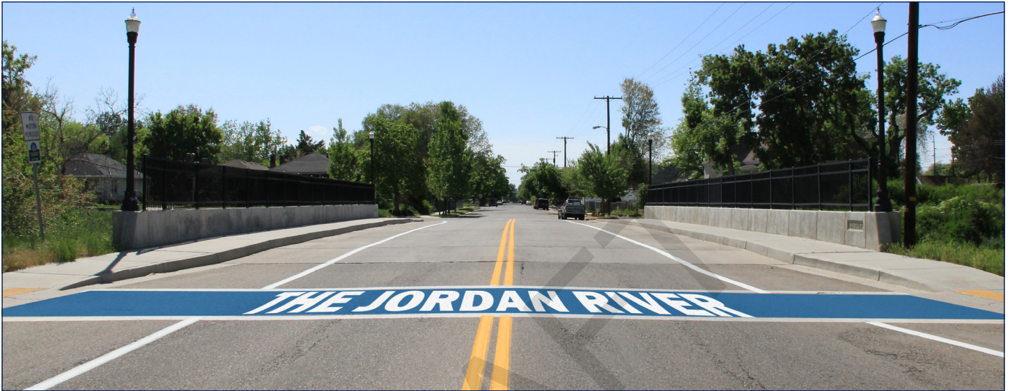
Something as simple as painting the Jordan River Parkway crosswalk can be an effective and relatively inexpensive way to make the river and pedestrians more visible.
